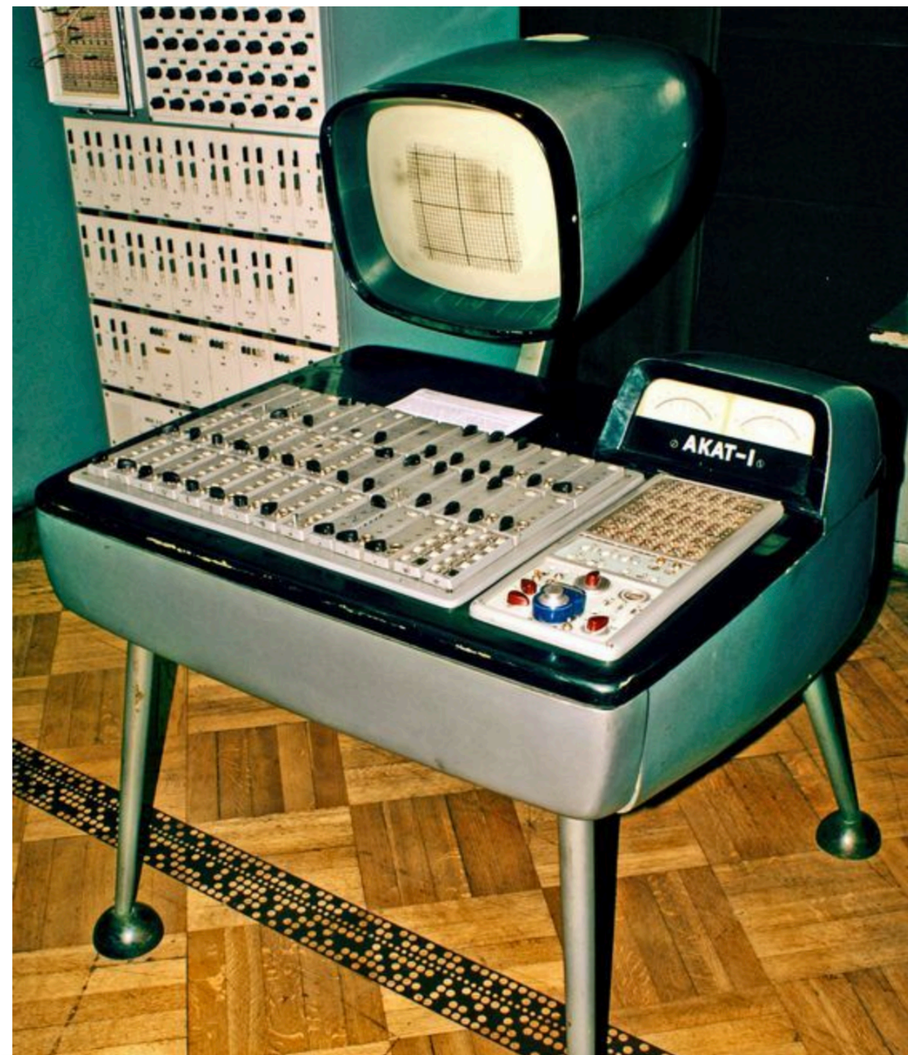
3. The AKAT-1, a Polish made analog computer from the 1960s
